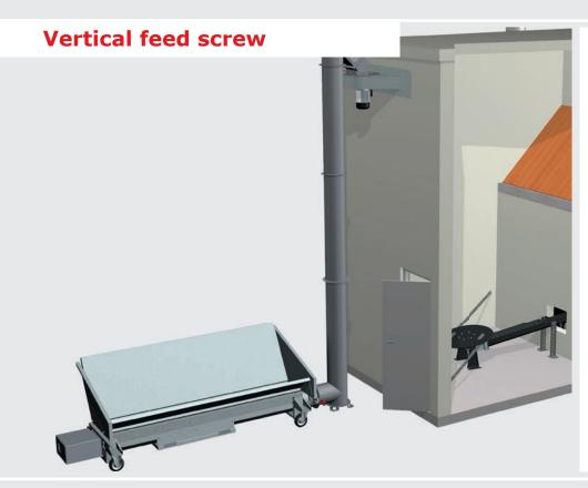
The vertical feed screw sets a new standard for feed output (45 m³/h), operating safety and bunker filling. The tipping gutter pushes the wood chips into the vertical feed system, which transports the fuel to the desired height for the centrifugal disc. Even distribution of the fuel is guaranteed as the vertical feed screw enables dust free filling of the fuel store.
